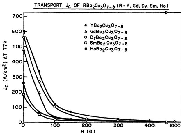
FIG. 2. Transport  $J_c$  at 77 K vs magnetic field for  $R\text{Ba}_2\text{Cu}_3\text{O}_{7-\delta}$  ( $R = \text{Gd, Dy, Sm, Ho, Y}$ ).
