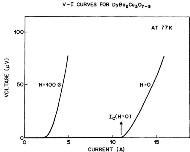
FIG. 3.  $V$ - $I$  curves for  $\text{DyBa}_2\text{Cu}_3\text{O}_{7-\delta}$  at 77 K indicating a critical current of 11 A at  $H=0$  and 2.4 A at  $H=100 \text{ G}$ .
