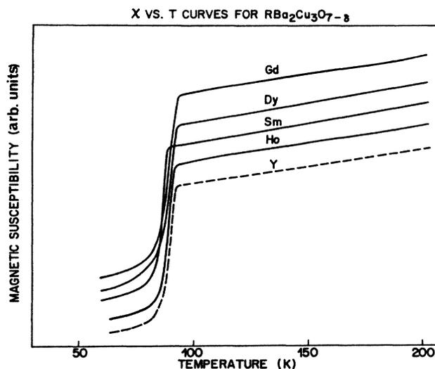
FIG. 1. Magnetic susceptibility vs temperature curves for  $\text{RBa}_2\text{Cu}_3\text{O}_{7-\delta}$  ( $R = \text{Gd, Dy, Sm, Ho, Y}$ ).
