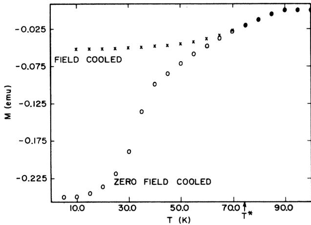
FIG. 1. Field-cooled and zero-field-cooled magnetization measurements of a  $\text{YBa}_2\text{Cu}_3\text{O}_7$  sample taken using a field of 500 G.
