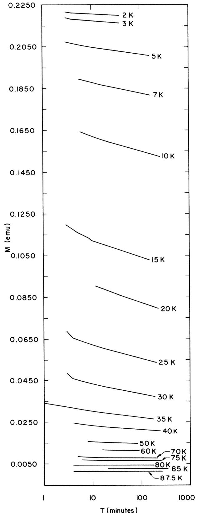
FIG. 2. Magnetization vs time of the sample studied in Fig. 1. Measurements were obtained by cooling in a field of 500 G and then removing the field. The residual magnetic field during these measurements was the order of 3 G.
