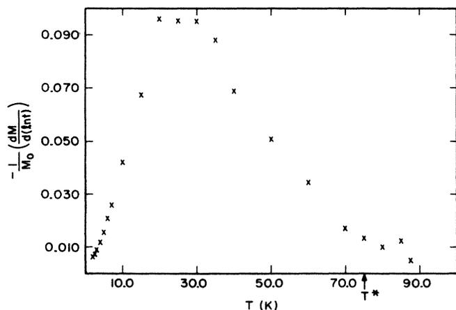
FIG. 3. Temperature dependence of the fractional change of the magnetization.  $M_0$  is the magnetization measured 1 min after the removal of the external magnetic field.
