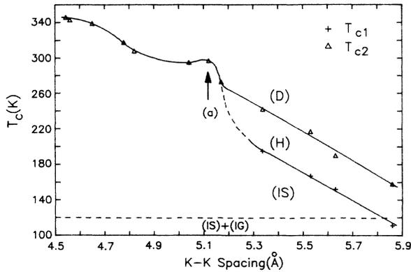
FIG. 5. Relationship between the transition temperatures as a function of the overlayer lattice parameter (K-K spacing). The dashed line at 120 K indicates  $T_{ca}$ . The K-K spacing can be converted to the coverage (Fig. 3). (a) indicates the value of K-K spacing for the  $(2 \times 2)$  structure. (IS) represents the incommensurate solid phase, (IG) the immobile gas, (H) the hexatic phase, and (D) the disordered phase.
