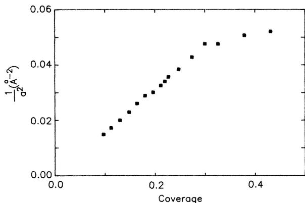
FIG. 3. Relationship between inverse square of the potassium nearest-neighbor spacing  $a$  and the potassium coverage on Cu(111) surface at 80K.
