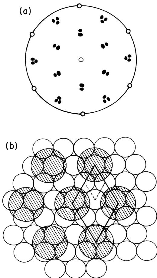
FIG. 1. (a) Schematic LEED pattern of the incommensurate phase at coverage of about 0.15 at 80 K. The extra beams are elliptical. (b) The structure of the potassium overlayer on Cu(111) of the incommensurate phase from (a). The solid and dashed lines indicate the overlayer and substrate surface unit cells, respectively.
