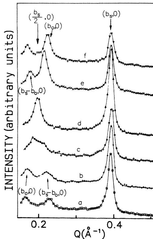
FIG. 2. The LEED beam's intensity profiles at  $E=92$  eV with the increase of the potassium coverage [(a)-(f)]: (a) for a weak incommensurate phase at coverage about 0.14; (d) for a clear  $(2 \times 2)$  phase at coverage about 0.25; (f) for a saturated incommensurate phase at coverage about 0.4. The substrate is at 80 K.  $b_s$  and  $b_0$  are the reciprocal-lattice constants of the substrate surface and the overlayer.
