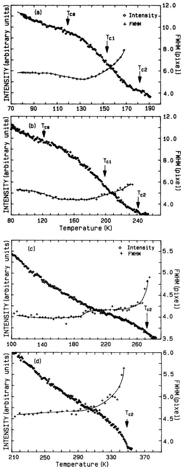
FIG. 4. Change of the LEED intensity and the beam width [FWHM is measured in  $(-b_0/2, b_0)$  direction] of the  $(b_0, 0)$  beam as a function of temperature after evaporation of potassium onto Cu(111) surface at 80 K. The overlayer lattice parameter is (a) 5.65 Å; (b) 5.33 Å; (c) 5.17 Å; (d) 4.54 Å. One pixel is equivalent to  $1.3 \times 10^{-2}$  of the reciprocal-lattice parameter ( $b_s$ ) in this measurement. The curves are to aid the eye in studying the data.
