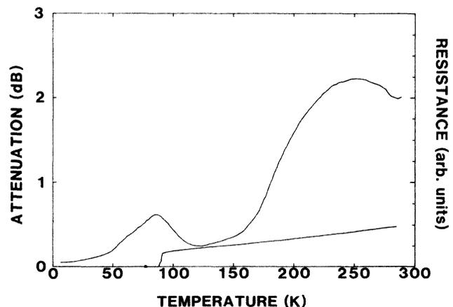
FIG. 1. The attenuation of 15 MHz longitudinal waves in a single-phased sample of  $\text{Y}_1\text{Ba}_2\text{Cu}_3\text{O}_7$  in the temperature range from 7 to 289 K. The lower curve represents values for resistance measurements.
