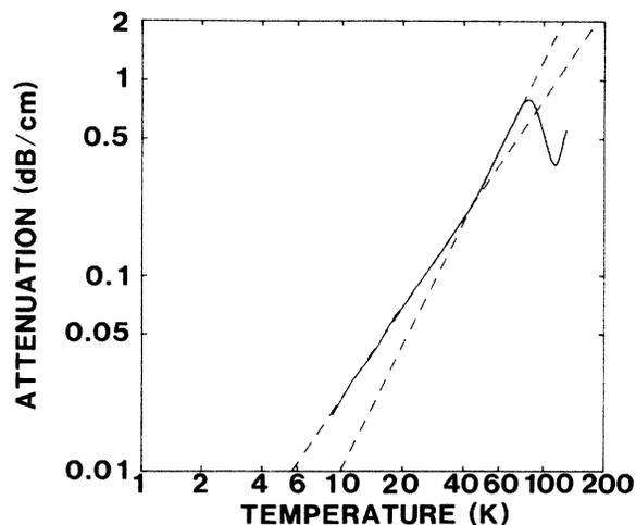
FIG. 3. Log-log plot of data in Fig. 2. The dashed lines yield  $T^n$  dependences in the superconducting state, where above 42 K  $n_1 = 2.1$  and below 42 K  $n_2 = 1.6$ .
