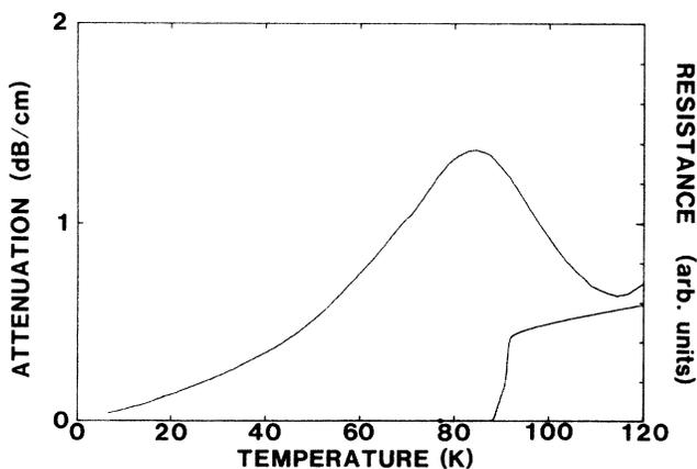
FIG. 2. Attenuation coefficient obtained during a different experimental run from the one displayed in Fig. 1 on the same sample of  $\text{Y}_1\text{Ba}_2\text{Cu}_3\text{O}_7$ . The temperature range covered was 7 to 120 K. The lower curve represents values for simultaneous resistance measurements.
