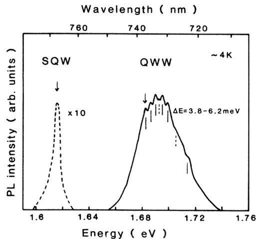
FIG. 1. Photoluminescence spectra measured at  $\sim 4$  K for QWW structure (solid line) and reference SQW only annealed without implantation (broken line). Solid bars indicate the position of clear peak structures and broken bars indicate indistinct ones. Downward arrows indicate the wavelength, where excitation spectra shown in Fig. 2 were measured.
