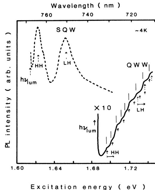
FIG. 2. Photoluminescence excitation spectra measured at  $\sim 4$  K for QWW structure (solid line) and reference SQW (broken line). The detection wavelength is denoted by upward arrow  $h\nu_{\text{lum}}$ . Solid bars above the spectrum of QWW indicate energy positions of the observed fine structures. Solid arrows and broken arrows under the spectrum QWW indicate calculated heavy-hole related and light-hole related transitions, respectively.
