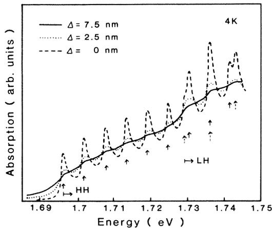
FIG. 4. Calculated absorption spectrum of QWW at 4 K under several degrees of inhomogeneity  $\Delta$  in the lateral width of QWW.
