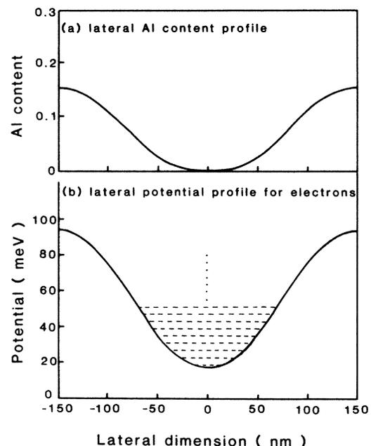
FIG. 3. Calculated lateral profile of (a) Al content along the center plane of SQW and (b) potential for electrons. Laterally quantized energy levels were calculated using Schrödinger equation and shown in (b) as broken lines.
