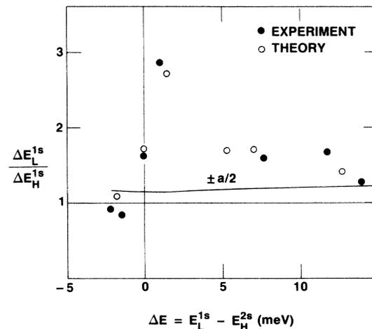
FIG. 3. The ratio  $R$  of the FWHM's of the  $1l/$  to the  $1h$  excitons as a function of the energy difference,  $\Delta E = E_L^{1s} - E_H^{2s}$ . The solid line is the calculated excess broadening of the  $1l/$  exciton with respect to the  $1h$  exciton due to quantum-well width fluctuations.
