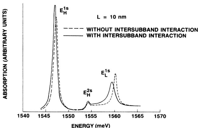
FIG. 1. Calculated absorption spectrum of a 10-nm GaAs/Al<sub>0.3</sub>Ga<sub>0.7</sub>As quantum well with (solid line) and without (dashed line) the intersubband interaction.
