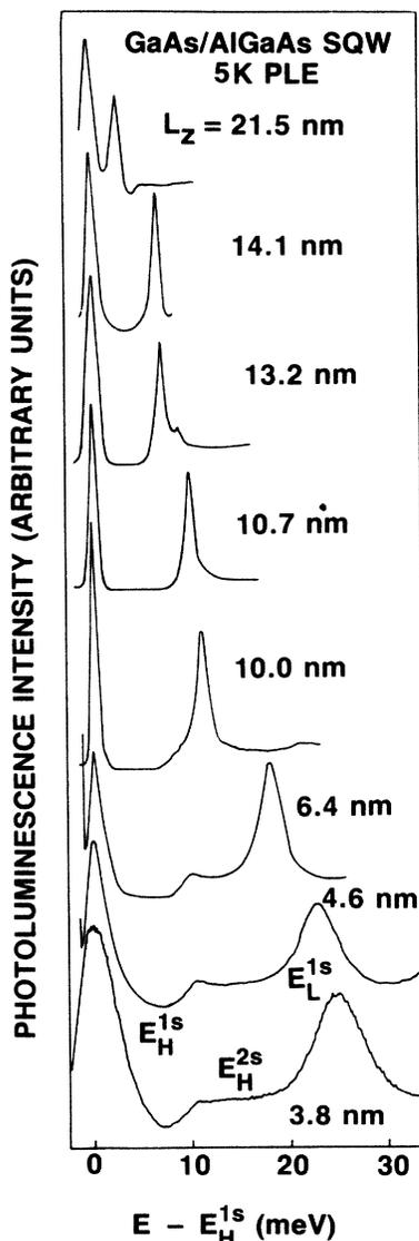
FIG. 2. Experimental low-temperature photoluminescence excitation spectra of several single GaAs/Al<sub>0.3</sub>Ga<sub>0.7</sub>As quantum wells with different well thicknesses. The horizontal energy scale for each spectrum was shifted so as to line up the  $E_H^1s$  peaks for easier comparison.
