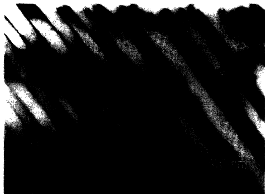
FIG. 1. Transmission electron micrograph of Y_1Ba_2Cu_3O_{7-\delta} showing twin boundaries imaged using (2\bar{1}3) planes. Upper portion of the figure is nearest to the foil edge.
