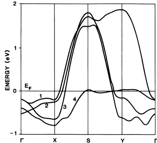
FIG. 2. Calculated band structure for  $\text{YBa}_2\text{Cu}_3\text{O}_7$ . Only the topmost bands are shown. The bands intersecting the Fermi level are labeled 1-4 (after Ref. 6).
