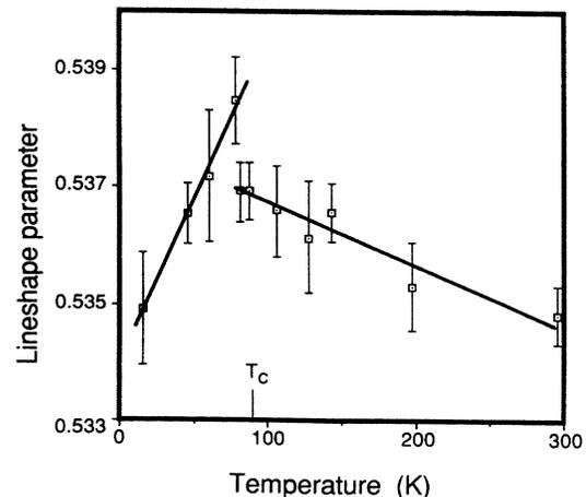
FIG. 1. Doppler-broadening line-shape parameter for  $\text{YBa}_2\text{Cu}_3\text{O}_{6.9}$  vs temperature.
