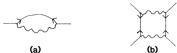
FIG. 5. Diagrams of (a) order w^2 contributing to r' and (b) w^4 contributing to u' . The wavy line indicates that this internal line contributes only the transverse part of the propagator and the solid internal line indicates only the longitudinal part of the propagator.
