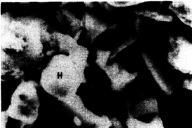
FIG. 7. Scanning electron micrograph of a portion of an  $\text{YBa}_2\text{Cu}_3\text{O}_7$  sample. Hash mark indicates  $0.1 \mu\text{m}$ .
