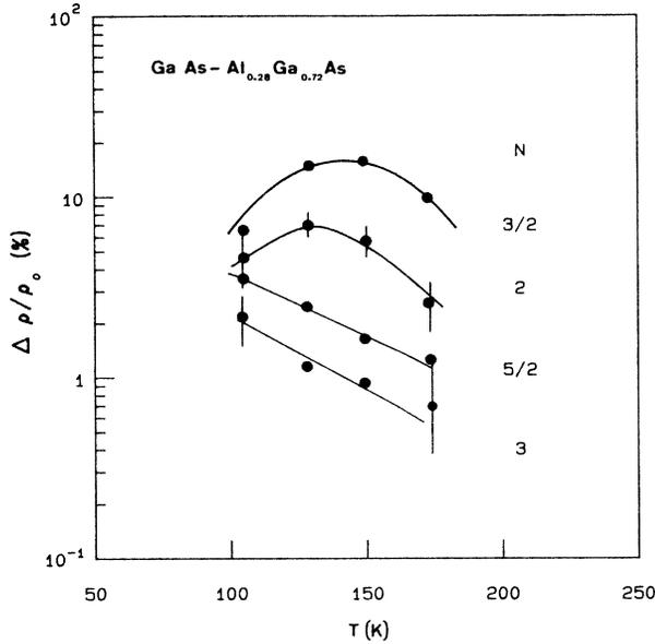
FIG. 6. Temperature dependence of the oscillation amplitude in GaAs-Al<sub>0.28</sub>Ga<sub>0.72</sub>As at ambient pressure. Only representative error bars are shown for clarity.
