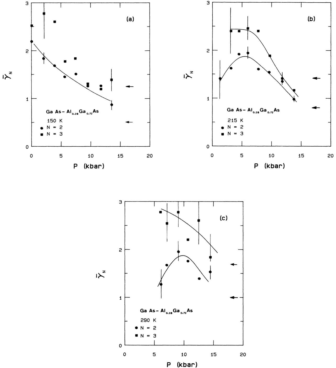
FIG. 9. Pressure dependence of the damping factor in GaAs-Al<sub>0.28</sub>Ga<sub>0.72</sub>As for two resonances, (a) at 150 K, (b) at 215 K, and (c) at 290 K. Arrows indicate the extreme values reported in literature for bulk GaAs (Refs. 28, 32, and 33). Lines are just guides for the eyes.
