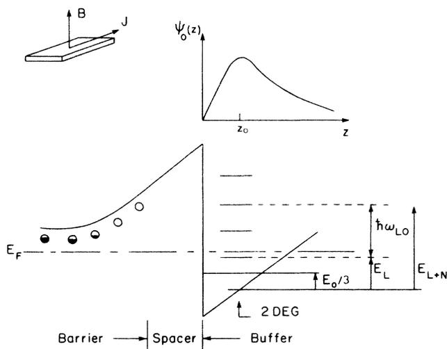
FIG. 4. Sketch of the energetic parameters for a resonant electron-LO-phonon coupling at a heterojunction interface.
