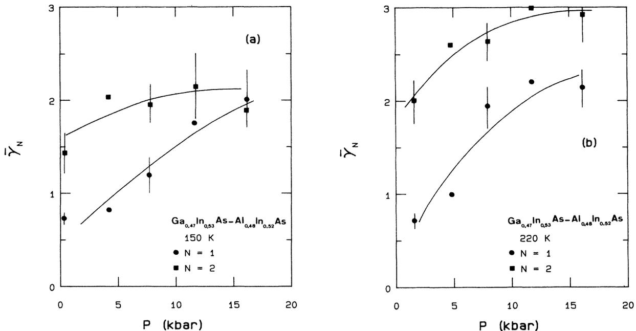
FIG. 10. Pressure dependence of the damping factor in  $\text{Ga}_{0.47}\text{In}_{0.53}\text{As}-\text{Al}_{0.48}\text{In}_{0.52}\text{As}$  for two resonances, (a) at 150 K and (b) at 220 K. Lines are just guides for the eyes.
