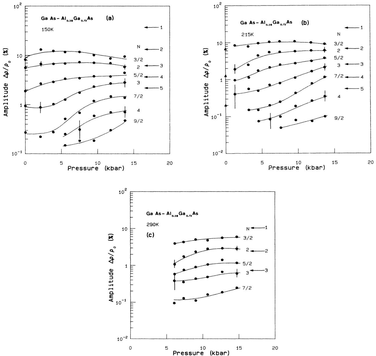
FIG. 7. Pressure dependence of the oscillation amplitude in GaAs- $\text{Al}_{0.28}\text{Ga}_{0.72}\text{As}$ , (a) 150 K, (b) at 215 K, and (c) at 290 K. Arrows indicate bulk amplitudes at ambient pressure after Kido and Miura (Ref. 33) and triangles at 0 kbar and 215 K are 2D amplitudes for  $N=1, 2$ , and 3 in a higher concentration heterojunction ( $N_s = 3.4 \times 10^{11} \text{ cm}^{-2}$ ) after Englert *et al.* (Ref. 6). Same remarks as in Fig. 6 apply for error bars in Figs. 7–10.
