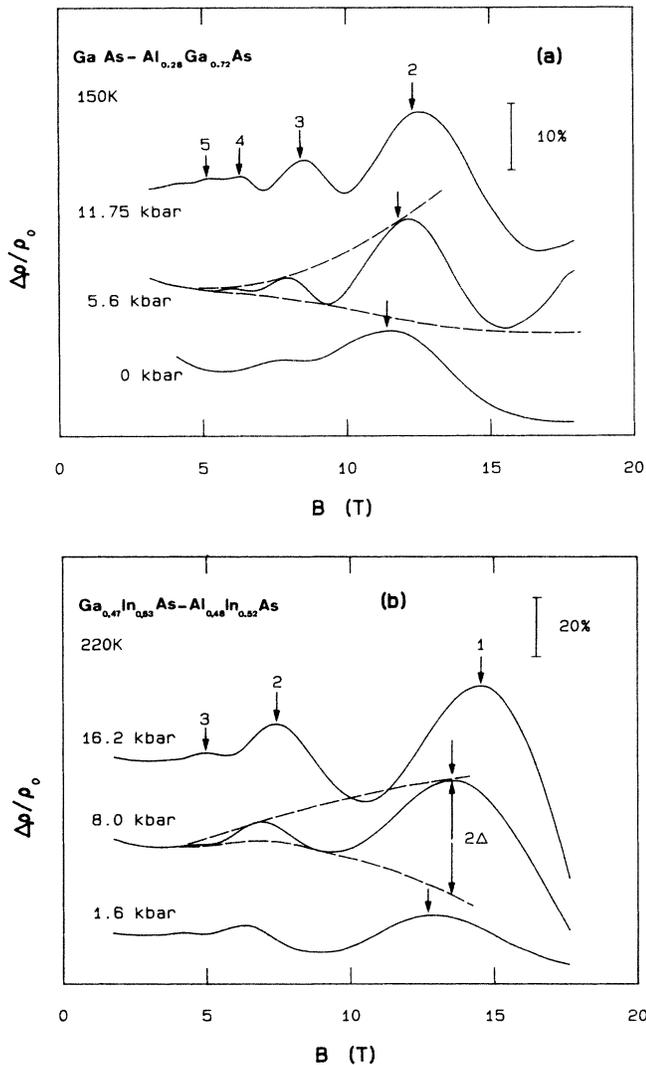
FIG. 1. Typical magnetophonon resonance oscillations for representative pressures: (a) in  $\text{GaAs-Al}_{0.28}\text{Ga}_{0.72}\text{As}$  at 150 K, and (b) in  $\text{Ga}_{0.47}\text{In}_{0.53}\text{As-Al}_{0.48}\text{In}_{0.52}\text{As}$  at 220 K. The dashed line shows the exponential damping of the oscillations,  $\Delta$  is the relative amplitude, and arrows point to the resonances.
