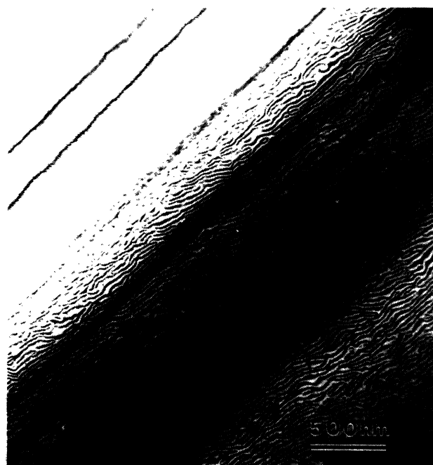
FIG. 1. Plan-view (220) two-beam bright-field TEM image of a \sim 70\text{-\AA} -thick \text{CoSi}_2 "substrate" layer. The dark bands crossing the figure diagonally are thickness fringes.
