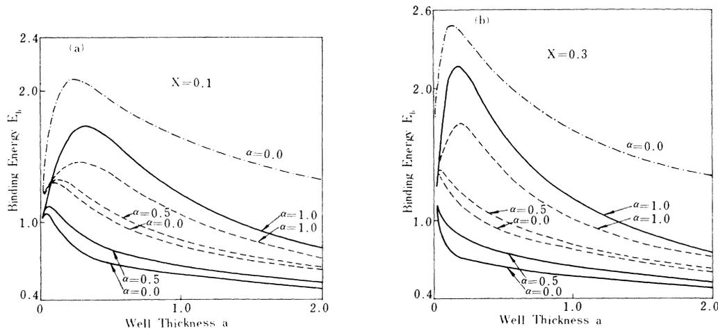
FIG. 2. Binding energy for the hydrogenic-donor ground state as a function of the GaAs layer thickness  $a$  for different  $\text{Ga}_{1-x}\text{Al}_x\text{As}$  layer thicknesses  $L$  and different impurity ratio positions,  $\alpha=2z_i/L$ . The solid, dashed, and dot-dashed curves are for barrier thicknesses  $L=2.0$ ,  $1.0$ , and  $0.0$ , respectively. (a) and (b) are for the alloy composition  $x=0.1$  and  $0.3$  of  $\text{Ga}_{1-x}\text{Al}_x\text{As}$ , respectively.
