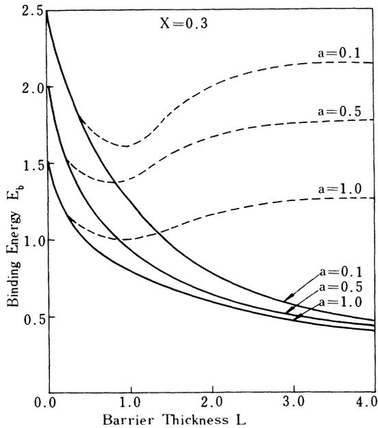
FIG. 3. Binding ground energy as functions of the  $\text{Ga}_{1-x}\text{Al}_x\text{As}$  layer thickness  $L$  for different well widths  $a$  and different impurity ratio positions  $\alpha$ . The solid and dashed curves are for the impurity on-center and on-edge, respectively.
