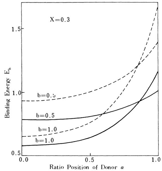
FIG. 4. Binding ground energy as functions of impurity ratio position for different well-barrier sizes. The solid and dashed curves are for the well thicknesses  $a=1.0$  and  $0.5$ , respectively.
