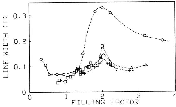
FIG. 3. Experimentally determined linewidth as a function of the filling factor for several samples: Sample 1 ( $\square$ ), sample 2 ( $\circ$ ), sample 3 ( $+$ ), and sample 4 ( $\triangle$ ).
