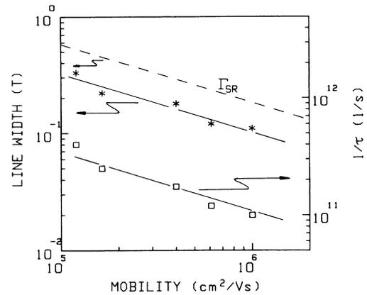
FIG. 6. CR linewidth values at  $\nu=2$  and fitting parameter  $1/\tau$  as a function of the zero-field mobility (samples 1–5). The slope of both lines is  $-\frac{1}{2}$ .  $\Gamma_{SR}$  is the CR linewidth for short-range scatterers predicted by the theory of Ref. 6.
