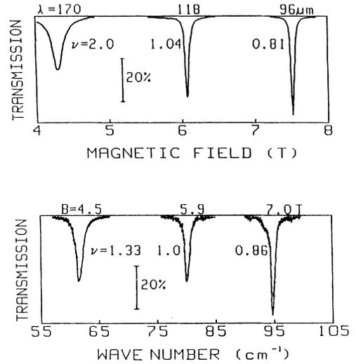
FIG. 2. Transmission spectra for sample 1, taken with the laser at the given wavelength ( $\lambda$ ) (top) and with the Fourier spectrometer at the given magnetic field ( $B$ ) (bottom) for different filling factors.
