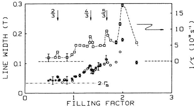
FIG. 4. CR linewidth vs filling factor for sample 1. The circles correspond to laser measurements, the asterisks to Fourier spectrometer data. The  $1/\tau$  data, obtained by fitting the experimental curves (see text), are characterized by squares. The dashed curve is for guiding the eye.  $2\Gamma_s$  indicates the saturation limited linewidth.
