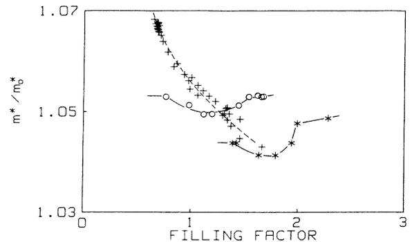
FIG. 5. The normalized CR mass ( $m_0^* = 0.065m_0$ ) as a function of the filling factor. The circles represent the data of the laser line with wavelength  $118.8 \mu\text{m}$ , the asterisks correspond to the  $170.6\text{-}\mu\text{m}$  line, and the crosses are the Fourier data.
