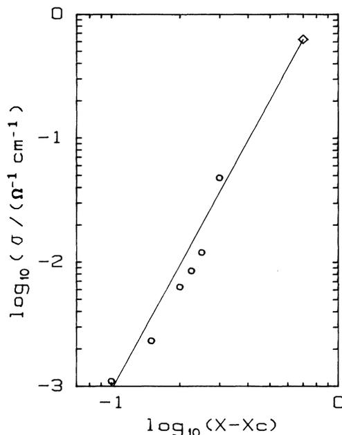
FIG. 2. A logarithmic plot of the dc conductivity at 298 K against  $(x - x_c)$  according to Eq. (1) for the AgI-AgPO<sub>3</sub> glasses,  $x_c = 0.3$ .  $\diamond$  represents an extrapolated value of  $\sigma_0$  for  $x = 1$ .
