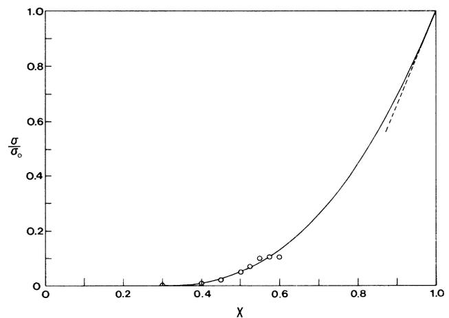
FIG. 1. A plot of the normalized dc conductivity at 298 K against the mole fraction of AgI for AgI-AgPO<sub>3</sub> glasses. Dashed line is the tangent on the curve as x → 1.
