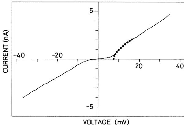
FIG. 1.  $I$ - $V$  characteristic of a superconducting-normal tunnel junction between a tungsten microprobe and a  $\text{La}_{1.85}\text{Sr}_{0.15}\text{CuO}_{4-\delta}$  sample. The solid dots are calculations using the BCS density of states and  $\Delta = 7.6$  meV.
