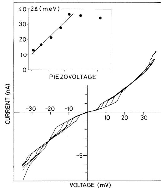
FIG. 3.  $I$ - $V$  curves for a normal-superconducting junction for different values of the pressure, exerted by the microprobe. The inset shows the energy gap  $2\Delta$  as a function of the voltage over the piezo, which is proportional to the force exerted by the tip.
