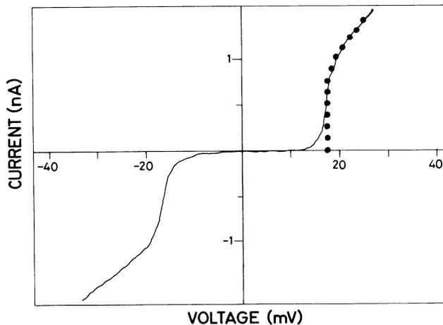
FIG. 2.  $I$ - $V$  characteristic of a superconducting-superconducting tunnel junction between two grains embedded in a  $\text{La}_{1.85}\text{Sr}_{0.15}\text{CuO}_{4-\delta}$  sample. The solid dots are calculations using the BCS density of states and  $\Delta = 8.7$  meV.
