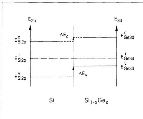
FIG. 2. A schematic diagram of the energy levels that were measured and used in the determination of the band lineup at an abrupt heterojunction interface.
