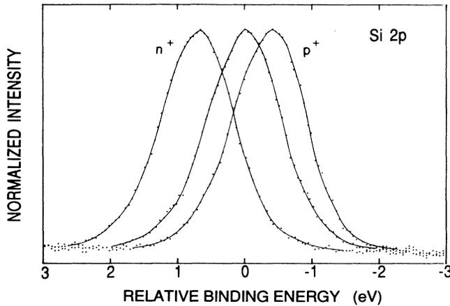
FIG. 3. Si 2*p* core-level spectra of the  $n^+$ -doped and  $p^+$ -doped reference samples with Sb and In overlayers, respectively. The middle spectrum is from the undoped Si/Si<sub>0.74</sub>Ge<sub>0.26</sub> heterostructure on Si.
