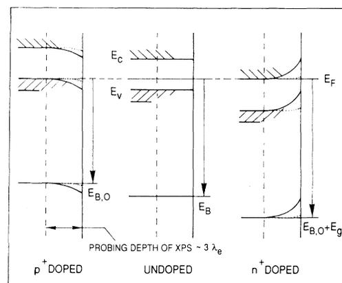
FIG. 1. Energy diagrams showing the energy levels near the surface of differently doped semiconductors. The dotted lines show schematically the reduction in band bending observed with In and Sb overlayers on  $p^+$  and  $n^+$  samples, respectively.
