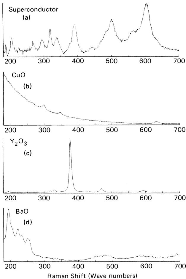
FIG. 2. Comparison of the background subtracted Raman spectrum of the superconductor (batch 1) to that of the various starting materials.
