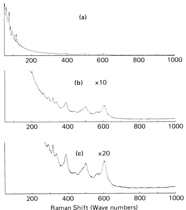
FIG. 1. Raman spectrum of the Y-Ba-Cu-O superconductor (batch 1) from 50 to 1000 cm<sup>-1</sup> with various scale expansions.
