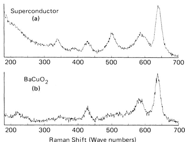
FIG. 4. Comparison of the Raman spectrum of the superconductor (batch 2) to that of the final product  $\text{BaCuO}_2$ .
