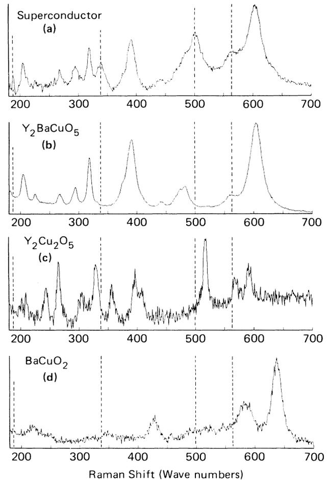
FIG. 3. Comparison of the background subtracted Raman spectrum of the superconductor (batch 1) to that of the various possible final products.
