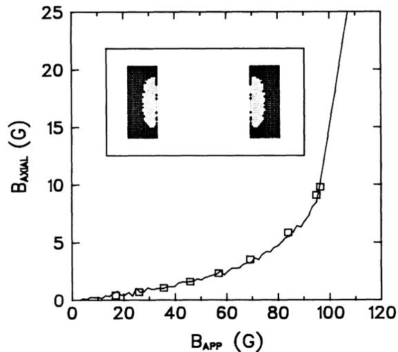
FIG. 4. An enlargement of the  $< 20$  K curve from Fig. 3. The boxes are from the model calculation described in the text with  $(J_c)_{fitted} = 500$   $A$   $cm^{-2}$ . The inset depicts the current distribution in the tube determined by our model calculation for a trapped field of 57 G. The dark area is the region where the current in the loops are at their saturation value and the light area shows the region where the loops carry zero current.
