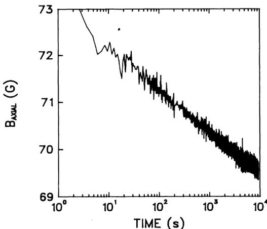
FIG. 2. Time dependence of the trapped magnetic field at 31 K (logarithmic scales).
