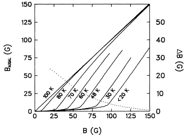
FIG. 3. The solid lines show the axial magnetic field (left scale) at the center of the tube as a function of the applied magnetic field ( $B_{app}$ ) after cooling to the indicated temperatures in zero applied field. The dots illustrate  $\Delta B \equiv B_{ext} - B_{axial}$  (right scale) vs  $B_{avg} \equiv (B_{ext} + B_{axial})/2$  at 70 K indicating the magnetic field dependence of the saturation current density  $J_c$ .
