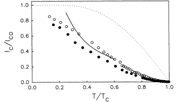
FIG. 4. Dependence of  $I_c/I_{c0}$  on  $T/T_c$  for sample A (open circles) and sample B (solid circles). Here  $I_{c0}$  is the extrapolated value of critical current at  $T=0$  K. The dotted curve represents calculation based on the Ambegaokar and Baratoff model (Ref. 18) for S-I-S junction; while the solid line represents normalized result obtained for de Gennes's model for proximity junction (Ref. 19) for temperatures lower than  $0.6T_c$ .
