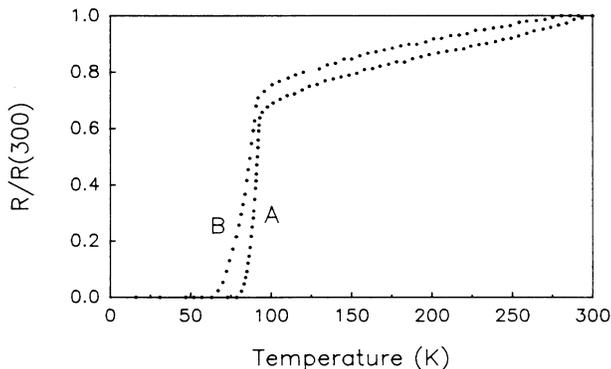
FIG. 1. Resistance-temperature relationships for two Y-Ba-Cu-O superconducting thin films (samples *A* and *B*) deposited on  $\text{SrTiO}_3(110)$  substrate.
