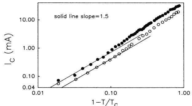
FIG. 3. Dependence of the critical current on  $1 - T/T_c$  for sample *A* (open circles) and sample *B* (solid circles).
