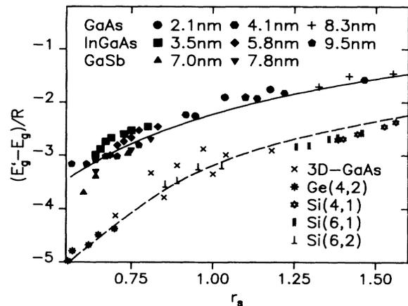
FIG. 3. Band-gap shift  $\Delta E_g$  scaled by the 2D and 3D Rydberg energies ( $R$ ) vs the dimensionless interparticle distance  $r_s$  for 2D and 3D structures. Si(4,1) denotes Si under high uniaxial stress parallel to the [110] (Ref. 15). The numerical result for a 2D plasma is calculated in a dynamical RPA with a single-plasmon pole approximation (full line). The universal 3D law (Ref. 3) is given by the dashed line.
