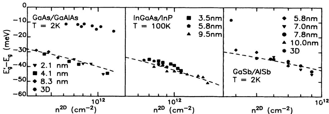
FIG. 2. Measured density dependence of the band renormalization for various MQW structures of the systems GaAs/Ga<sub>1-x</sub>Al<sub>x</sub>As,  $\text{In}_x\text{Ga}_{1-x}\text{As}/\text{InP}$ , and GaSb/AlSb as well as for bulk GaAs (Ref. 2) and bulk GaSb (Ref. 14). The density axes for the 2D and 3D cases are based on the interparticle distance. The 2D band renormalization depends in all systems on the density proportional to  $n^{1/3}$  as expected theoretically (Ref. 13) (dashed lines).
