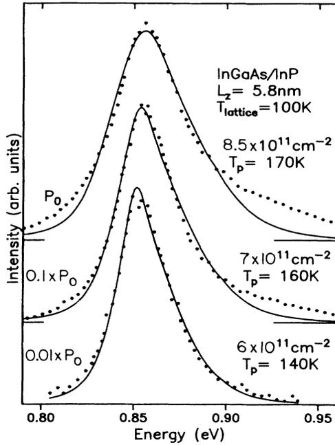
FIG. 1. Luminescence spectra and line-shape fits (solid lines) for an  $\text{In}_x\text{Ga}_{1-x}\text{As}/\text{InP}$  sample of  $L_z = 5.8$  nm as a function of the excitation intensity ( $P_0 \approx 500$  kW/cm<sup>2</sup>).
