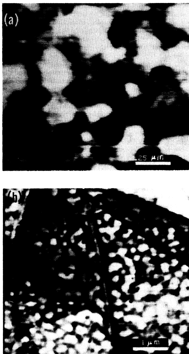
FIG. 1. Dark-field STEM image taken using the elastically scattered electrons. (a) The full scale of the image is 1.4 \mu\text{m} and demonstrates the presence of small islands of rubidium formed within the graphite host. (b) The full scale of the image is 5.6 \mu\text{m} . The dark lines are the boundaries of the HOPG domains.
