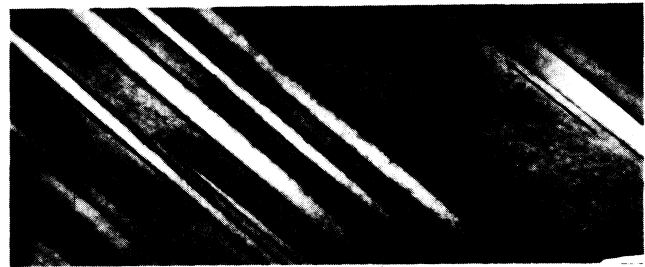
FIG. 1. Transmission electromicrograph YBa_2Cu_3O_x polycrystal. The parallel domains here are on the average \sim 1000 Å apart, and aligned along [110] direction. The interfaces are seen edge on. The orthorhombic a and b axes are found to alternate along these interfaces.
