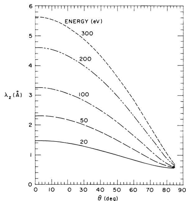
FIG. 4. Calculated positron penetration depths  $\lambda_z$  vs polar angle  $\theta$  for various energies (eV). Sample is Cu(100).
