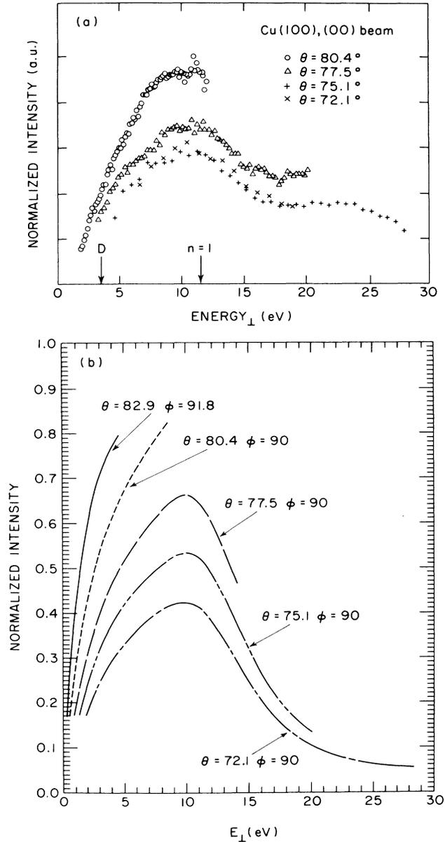
FIG. 3. (a) Experimentally observed normalized specular LEPD from Cu(100) for various polar beam angles as denoted in the figure. First-order Bragg peak indicated by arrow below  $n=1$  and position of dipole potential  $D$  is also displayed. (b) Calculated specular LEPD from Cu(100) for various polar beam angles using the quasikinematic model.
