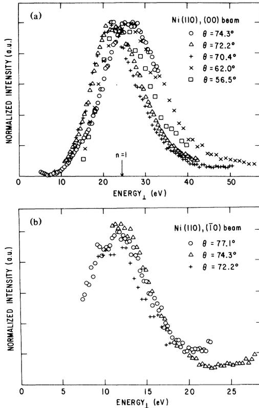
FIG. 2. (a) Normalized specular LEPD from Ni(110) plotted as a function of  $E_{\perp}$  (projected energy along surface normal) for various incident polar angles as denoted in the figure. All intensities rescaled to a common peak value. First-order Bragg peak denoted by arrow. (b) Similar plot for  $(\bar{1},0)$  beam.
