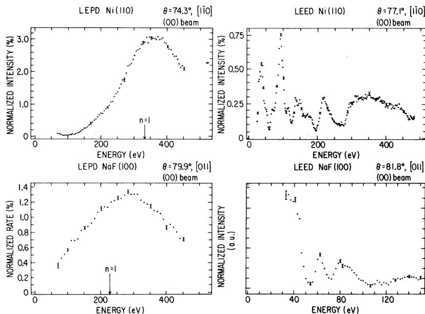
FIG. 1. Comparison of normalized specular LEPD and LEED spectra from NaF(100) and Ni(110). The arrow below  $n=1$  denotes the first-order Bragg peak position.
