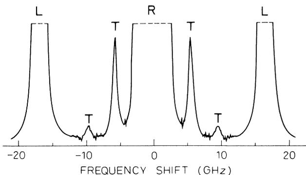
FIG. 2. Brillouin spectrum of fcc  $\text{Li}_2\text{SO}_4$  at 938 K; *R*, *L*, and *T* are Rayleigh, longitudinal Brillouin, and transverse Brillouin components, respectively.
