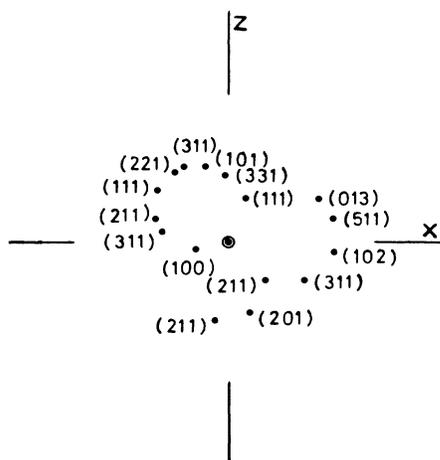
FIG. 1. Laue diffraction spots identified by their Miller indices of a fcc  $\text{Li}_2\text{SO}_4$  single crystal. The Euler angles ( $\Psi, \Theta, \Phi$ ) are  $\Psi=66.5^\circ$ ,  $\Theta=39.0^\circ$ , and  $\Phi=107.0^\circ$ . The  $x$  axis represents the direction of the polarization of the incident beam, the  $y$  axis (into the paper) represents the direction of the scattered light, and the  $z$  axis represents the direction of the incident laser beam.
