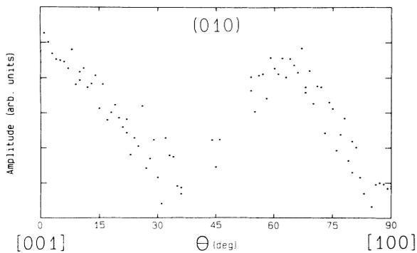
FIG. 2. The de Haas-van Alphen amplitude for the fundamental harmonic in platinum diluted with iron as a function of magnetic field direction, with the magnetic field in the (010) plane. A spin-splitting zero is located at  $\theta=33^\circ$ , to be compared with pure Pt which has no spin-splitting zeros for the fundamental.
