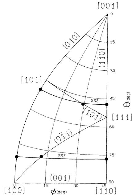
FIG. 1. The basic irreducible  $\frac{1}{16}$  wedge for the  $X$  pocket centered at  $00\frac{1}{2}$ , with the two spin-splitting-zero contours for the second harmonic (solid lines) displayed. The solid circles indicate the detected SSZ's. The SSZ's in the nonsymmetry planes are measured with less accuracy.
