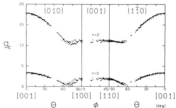
FIG. 4. The values of  $g_c(\theta, \phi)$  in the symmetry planes on the  $X$  pocket calculated from  $R(\theta, \phi)$  with  $n=0$  and  $n=2$ , using the effective electron masses from KW.
