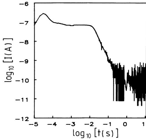
FIG. 1. The transient photocurrent of a sample made from a benzotriazole derivative (20 wt.%) and bisphenol-A-polycarbonate, measured by the time-of-flight technique (sample thickness  $d = 10 \mu\text{m}$ , applied voltage  $U = 300 \text{ V}$ , temperature  $T = 333 \text{ K}$ ).
