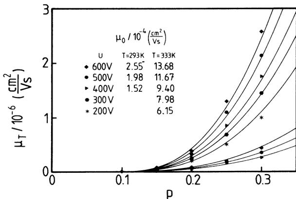
FIG. 2. The effective mobilities  $\mu_T$  as a function of the benzotriazole concentration  $p$ . The  $\mu_T$  data were measured at the  $U$  and  $T$  values given in the inset. All curves are fits to the percolation model, Eq. (1), with  $p_c = 0.1$  and  $\bar{i} = 2.5$ . The resulting  $\mu_0$  values are listed in the inset.
