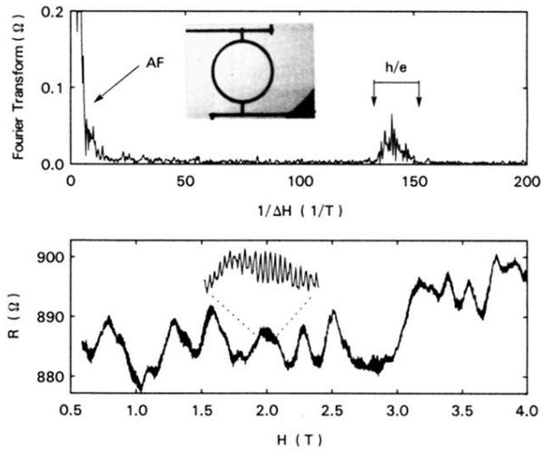
FIG. 1. The magnetoresistance  $R(H)$  at  $T=0.06$  K in sample 1 (the inset illustrates the  $h/e$  oscillations which pervade the entire field range) and the Fourier transform of  $R(H)$  (inserted is a photograph of sample 1).
