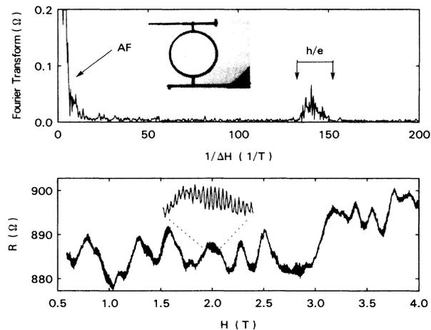
FIG. 1. The magnetoresistance  $R(H)$  at  $T=0.06$  K in sample 1 (the inset illustrates the  $h/e$  oscillations which pervade the entire field range) and the Fourier transform of  $R(H)$  (inserted is a photograph of sample 1).
