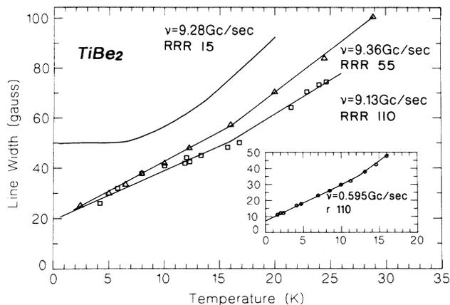
FIG. 3. Linewidth as a function of temperature as  $X$  band for the 15, 55, and the 110 RRR samples. The results of the 15 and 55 RRR samples are from earlier publications (Refs. 7 and 9, respectively). The inset show the linewidth at 0.595 Gc/sec for the RRR 110 sample.
