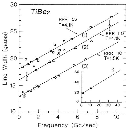
FIG. 1. Linewidth as a function of the frequency for the 55 and 110 RRR samples at 4.1 K and for the 110 RRR sample at 1.5 K, between 0.5 and 10 Gc/sec. The inset shows the linewidth of the RRR 110 sample at 4.1 K between 0.5 and 10 Gc/sec, together with the measurement at 35.6 Gc/sec; the straight line is extrapolated from the low-frequency results.
