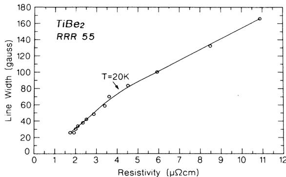
FIG. 4. Linewidth as a function of the resistivity for the 55 RRR sample, the temperature being the implicit parameter. The results are from an earlier publication (Ref. 9).
