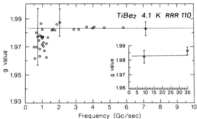
FIG. 2.  $g$  value as a function of frequency of the 110 RRR sample at 4.1 K between 0.5 and 10 Gc/sec. The inset includes the result at 35.6 Gc/sec.
