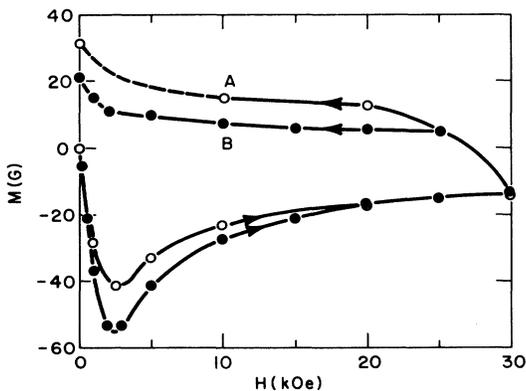
FIG. 2. The magnetic moment in gauss vs the applied field in kOe at 4.4 K for polycrystalline samples A and B.
