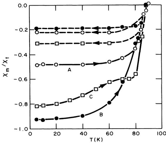
FIG. 1. Normalized volume susceptibility  $\chi_m$  (measured) divided by  $\chi_t$  (theory) vs temperature for the three polycrystalline samples A, B, and C (see Table I). The measurements made in increasing temperature gives the diamagnetic shielding while those for decreasing temperature gives the Meissner effect. The applied field is  $H = 14$  Oe.
