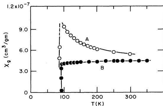
FIG. 5. The gram susceptibility of samples *A* and *B* as a function of temperature above the superconducting transition temperature.
