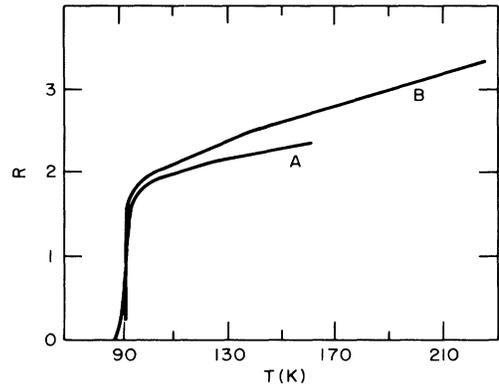
FIG. 6. Resistance in arbitrary units as a function of temperature for samples *A* and *B*. At 150 K the absolute values of resistivity is  $1.68 \text{ m}\Omega\text{cm}$  for sample *A* and  $1.97 \text{ m}\Omega\text{cm}$  for sample *B*.
