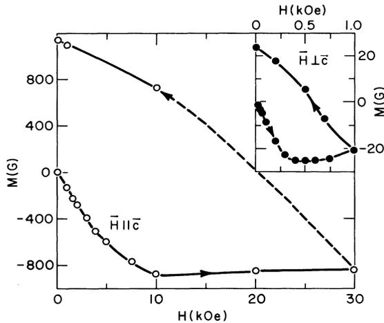
FIG. 4. Magnetic moment in gauss of the single crystal as a function of magnetic field at a temperature of 4.5 K. The main plot is for  $H$  parallel to the  $c$  axis of the crystal while the inset plot is for  $H$  perpendicular to the  $c$  axis.
