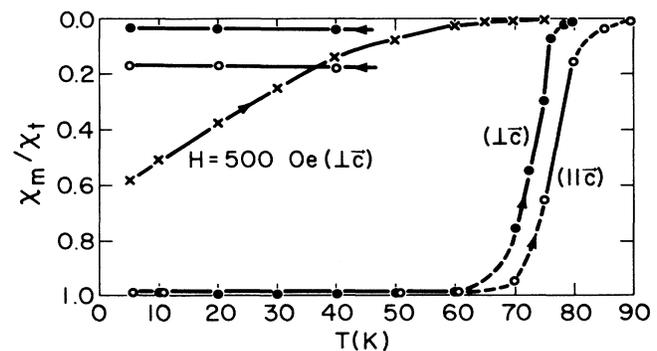
FIG. 3. The normalized susceptibility for the single crystal parallel and perpendicular to the  $c$  axis at an applied field of 14 Oe. The data points marked with an  $\times$  are for an applied field of  $H = 500$  Oe with the field perpendicular to the  $c$  axis of the crystal.
