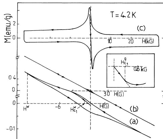
FIG. 1. The isothermal magnetization (4.2 K) as a function of field for three different field scales. Note the presence of two very different regimes of irreversibilities near (a) and (b)  $H = 0$  and (c) at much higher fields.
