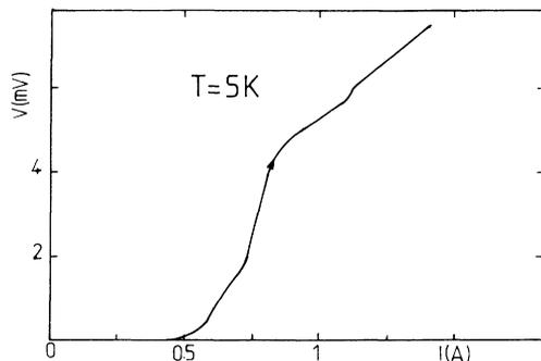
FIG. 5. The voltage-current characteristic at about 5 K. Note that the samples corresponding to Figs. 4 and 5 have been cut from the same ingot but have different geometrical factors.
