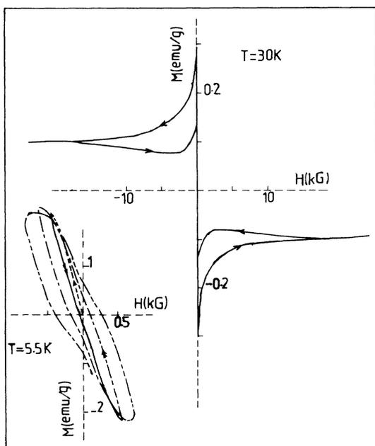
FIG. 2. The magnetization as a function of field at 30 K. The inset shows an example of magnetic irreversibilities at 5.5 K.
