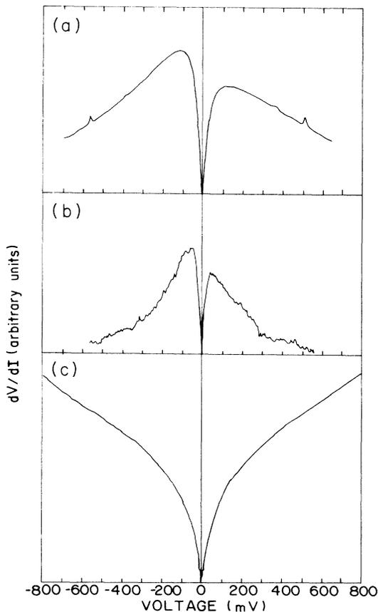
FIG. 2. Differential resistance ( $dV/dI$ ) measured at 10.3 K, (a) from a granular sample of Y-Ba-Cu-O in the direction parallel to the disk faces, (b) from the same granular sample as (a) but in the direction perpendicular to the disk faces, and (c) from a homogeneous sample of Y-Ba-Cu-O in the same conditions as (a).
