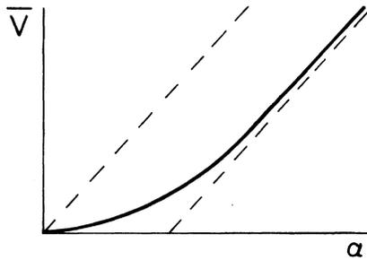
FIG. 6. Voltage-current characteristic for following the two-band picture. The relaxation time  $\tau$  is assumed to be independent of both current and energy.
