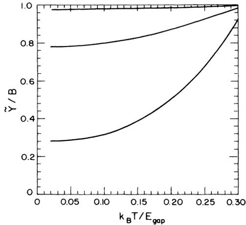
FIG. 4. Correction to the bare Zener probability  $\tilde{Y}/B$  vs the normalized temperature  $k_B T/E_{\text{gap}} = k_B T/2\Delta$  for various values of dissipation,  $\eta$ . The current is chosen such that  $\Delta^2/\alpha = 5$ .
