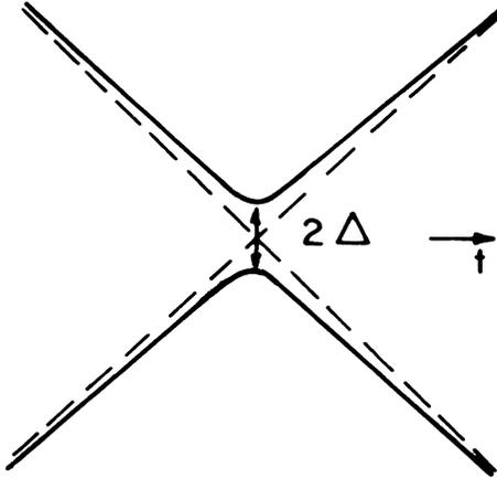
FIG. 3. Energy levels of the decoupled system as function of time (schematic).
