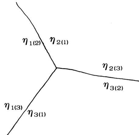
FIG. 2. Values of the order parameters at the grain boundaries.
