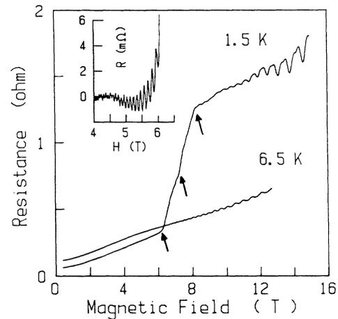
FIG. 1. Magnetoresistance of  $(\text{TMTSF})_2\text{ClO}_4$  in the very relaxed state. At 1.5 K, the SDW threshold appears at 6 T, followed by the FISDW transitions (arrows). The oscillatory resistance is seen to be enhanced above 10 T. Inset shows the oscillations below the threshold field. For  $T=6.5$  K,  $H_t > 15$  T.
