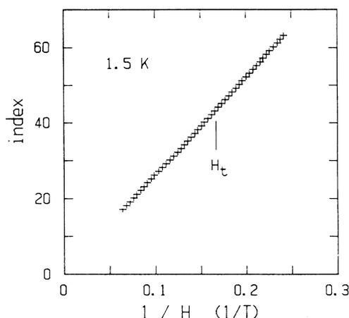
FIG. 3. Indexed peaks vs  $1/H$ , from resistance data at 1.5 K, giving the SdH\* frequency.  $H_c$  marks the FISDW threshold.
