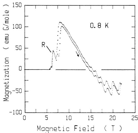
FIG. 4. Magnetization in very relaxed state, showing FISDW transitions and dHvA-type oscillations.  $R$  marks the extra step corresponding to the Hall sign reversal.
