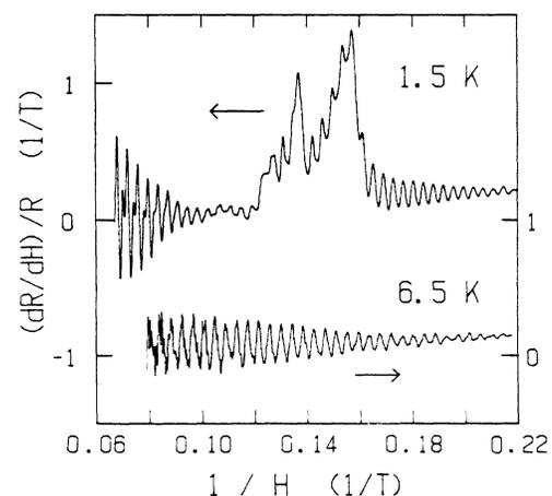
FIG. 2. The logarithmic derivative of the resistance vs inverse field, showing oscillations at all field values.
