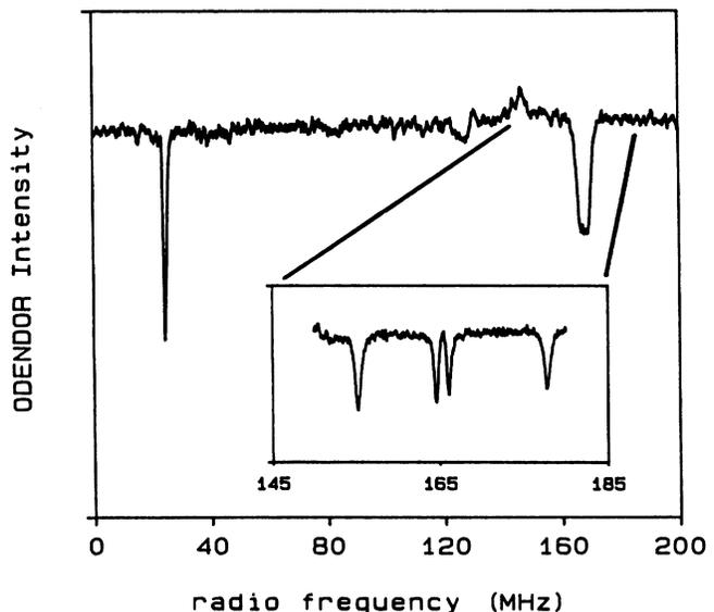
FIG. 3. The ODENDOR spectrum of the P<sub>In</sub> antisite with  $\mathbf{B} \parallel [100]$  at  $B = 1.19 \text{ T}$  and  $T = 1.7 \text{ K}$ . The inset shows the P lines with  $\mathbf{B} \parallel [100] + 10^0$ .
