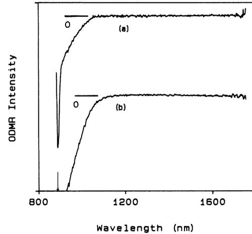
FIG. 2. The spectral dependence (corrected for detector and monochromator responses) of the P<sub>In</sub> antisite ODMR spectrum: (a) as-grown sample, (b) electron-irradiated sample. The band gap of InP is indicated by an arrow.
