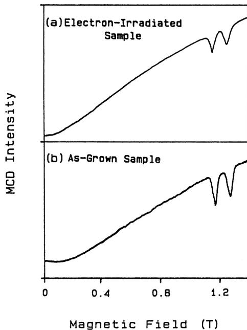
FIG. 1. The ODMR spectrum of the P<sub>In</sub> antisite in InP with  $\mathbf{B} \parallel [100]$  at  $T = 1.7 \text{ K}$  and  $\nu = 35.0 \text{ GHz}$ . The gain for (b) has been increased by a factor of 4.
