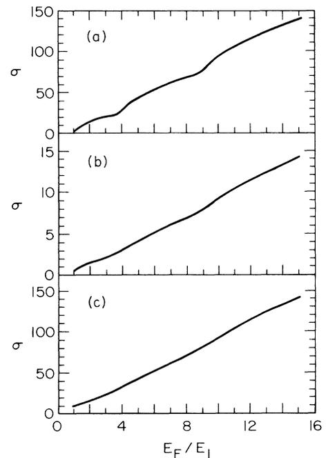
FIG. 2. Calculated conductivity in the 1D system corresponding to Fig. 1 as a function of  $E_F/E_1$  for different values of level broadening ( $\Gamma$ ) and temperature ( $T$ ): (a)  $\Gamma = 0.15$  meV and  $T = 1.2$  K, (b)  $\Gamma = 1.52$  meV and  $T = 1.2$  K, (c)  $\Gamma = 0.15$  meV and  $T = 10$  K. Only intrasubband scattering (due to short-range scatterers) is included. Same absolute units are used in (a)–(c).
