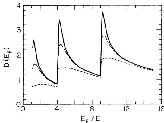
FIG. 1. Impurity-broadened density of states  $D(E_F)$  in a model 1D system (infinite square-well confinement with width  $= 500$  Å) for three different values of the level broadening  $\Gamma = 0.15$  (solid line),  $0.38$  (dash-dotted line),  $1.52$  (dashed line) meV. The Fermi energy is measured in the units of the ground subband bottom  $E_1 = 0.79$  meV.
