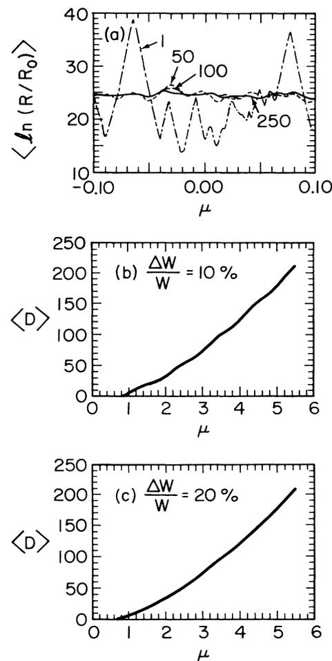
FIG. 4. (a) Calculated average fluctuating resistance  $\langle \ln R \rangle$  in a *finite* 1D chain as a function of the chemical potential for various numbers of parallel inversion lines as noted (see Refs. 3 and 5), (b) calculated conductivity  $D$  for 250 parallel inversion lines (for parabolic potential confinement) with width fluctuations of 10%, and (c) of 20%. [ $\Gamma/E_1 = 0.1$  for (b) and (c).]
