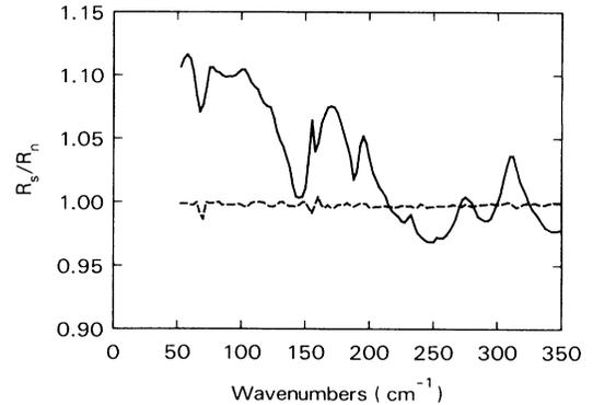
FIG. 3. We show the normalized reflectance  $R_s/R_n$  between the superconducting (13 K) and normal (93 K) states of the Y-Ba-Cu-O composition sample A as a function of frequency (solid line). Also shown is the reflectivity ratio for two runs taken at 93 K (dashed curve).
