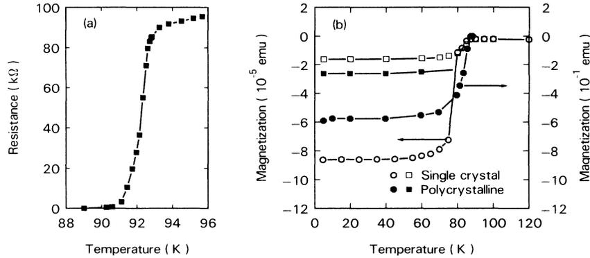
FIG. 1. (a) Resistive transition for the polycrystalline single-phase sample A, and (b) magnetic-susceptibility measurements for the polycrystalline single-phase sample A and the single-crystal sample B. In (b) the circles were taken while warming the sample and the squares were taken in the subsequent cooldown.
