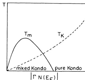
FIG. 6. Schematic dependence of the Kondo temperature,  $T_K$ , and magnetic ordering temperature,  $T_m$ , on the interaction strength  $|\Gamma N(E_F)|$  after Ref. 18.
