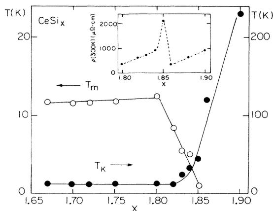
FIG. 5. Kondo temperature,  $T_K$  (●), and magnetic ordering temperature,  $T_m$  (○), vs composition for alloys in the system  $\text{CeSi}_x$ . Inset shows the room temperature resistivity for the tetragonal alloys.
