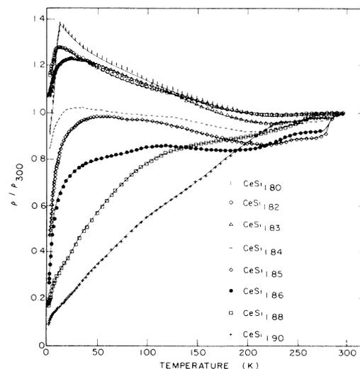
FIG. 3. Electrical resistivity normalized to the value at room temperature as a function of temperature for eight alloys in the system  $\text{CeSi}_x$ .
