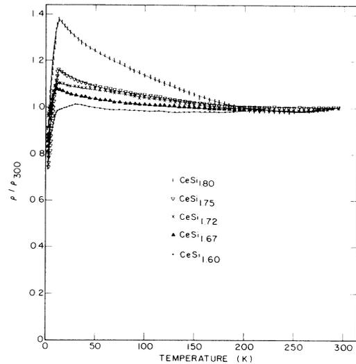
FIG. 2. Electrical resistivity normalized to the value at room temperature as a function of temperature for five alloys in the system  $\text{CeSi}_x$ .
