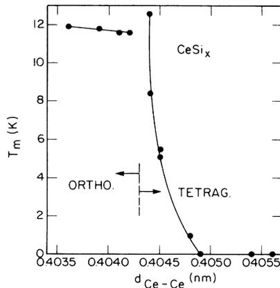
FIG. 4. Magnetic ordering temperature, *T<sub>m</sub>* vs the shortest Ce-Ce separation distance.
