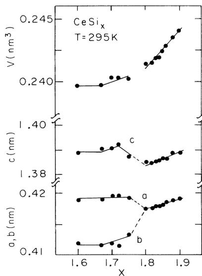
FIG. 1. The room temperature lattice parameters and unit-cell volume for alloys in the series  $\text{CeSi}_x$ .
