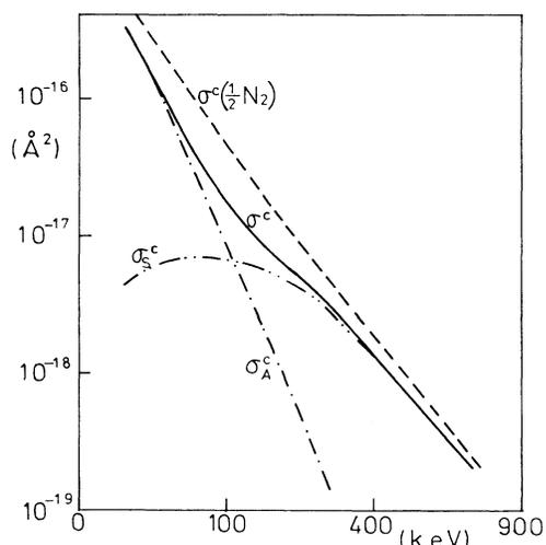
FIG. 1. Shell,  $\cdots$ , Auger,  $-\cdot-$ , and total  $\text{---}$ , capture cross section for  $\text{H}^+$  colliding with Al. For comparison, we show the capture cross section (normalized to one atom of the target) for the gas collision  $\text{H}^+-\text{N}_2$ ,  $\cdots$ .
