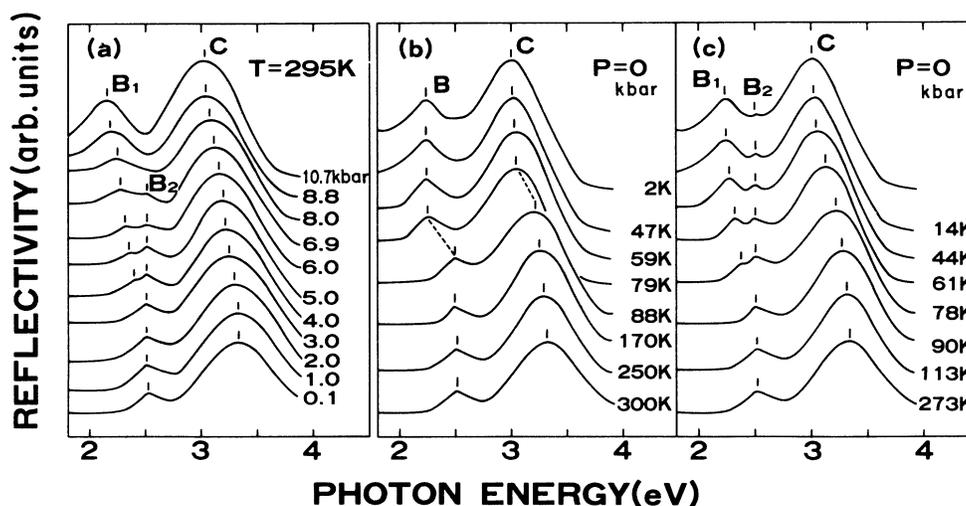
FIG. 2. Optical reflectivity spectra of TTF-*p*-chloranil crystal as a function of pressure at 295 K in (a), and as a function of temperature at  $P=0$  kbar on pure crystal and impurity (7 mol % trichloro-*p*-benzoquinone)-doped crystals in (b) and (c), respectively. The spectra in (b) and (c) were taken from Refs. 4 and 6.
