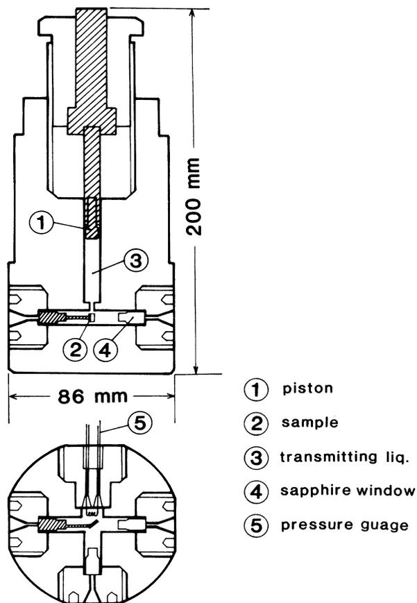
FIG. 1. High-pressure optical cell used in the study.
