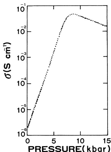
FIG. 3. Electric conductivity of TTF-*p*-chloranil crystal along the  $a$  axis (the stack axis) as a function of pressure at 295 K.
