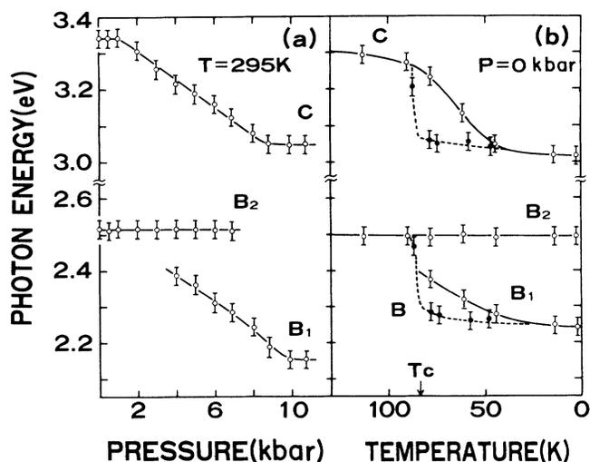
FIG. 4. Peak energies of intramolecular excitation bands in TTF-chloranil crystals (a) as a function of pressure at 295 K and (b) as a function of temperature at  $P=0$ . Solid and open circles in (b) represent the experimental points for pure and impurity (7 mol % trichloro-*p*-benzoquinone)-doped crystal, respectively. The data in (b) were taken from Refs. 4 and 6.
