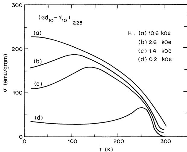
FIG. 2. The temperature dependence of the magnetic moment of the  $(10,10)$  superlattice in a series of applied fields.
