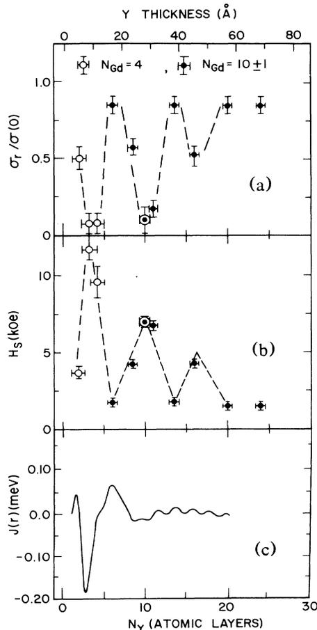
FIG. 4. The oscillatory dependence of (a)  $\sigma_r/\sigma(0)$ , and (b)  $H_s$ , on  $N_Y$  in two series of superlattices with  $N_{\text{Gd}} = 4$ , and  $N_{\text{Gd}} = 10 \pm 1$ . The dashed lines are to guide the eyes. (c) The calculated functional dependence of  $J_{\text{Gd-Y}}(r)$  on  $N_Y$ .
