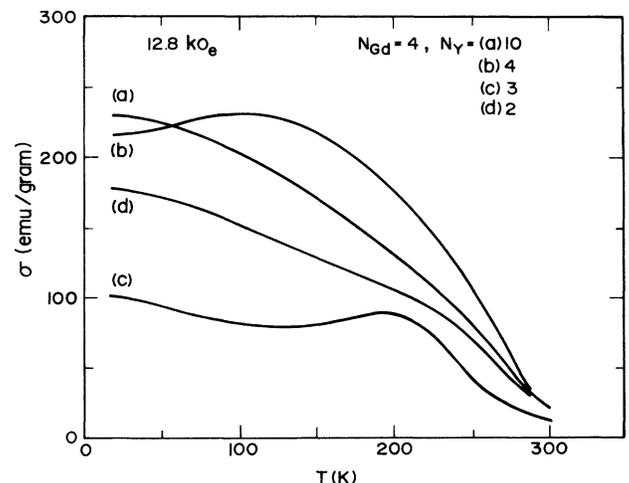
FIG. 3. The temperature dependence of the magnetic moment of the  $(4,2)$ ,  $(4,3)$ ,  $(4,4)$ , and  $(4,10)$  superlattices in an applied field of 12.8 kOe.
