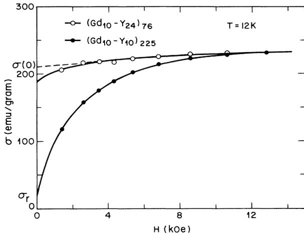
FIG. 1. The in-plane magnetization curves at 12 K for the  $(10,10)_{225}$  and  $(10,24)_{76}$  superlattices.
