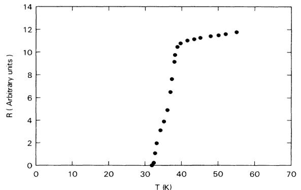
FIG. 1. Resistance vs temperature for a sample of  $\text{La}_{1.8}\text{Sr}_{0.2}\text{CuO}_{4-y}$  (sample a), from the same batch as that used for the tunneling measurements. The measuring current density was 0.01 A/cm<sup>2</sup>.
