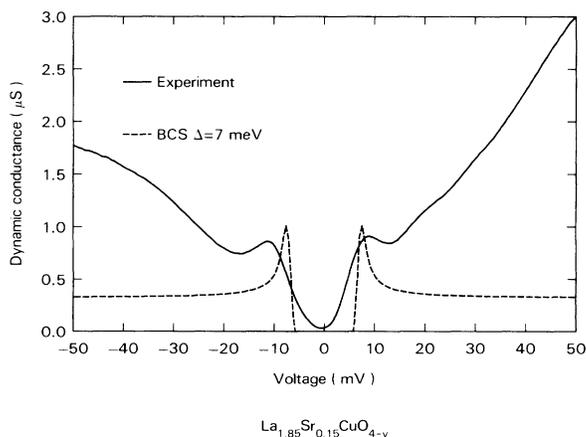
FIG. 3. Dynamic conductance vs voltage for tunneling from a PtIr tip into a sample of  $\text{La}_{1.85}\text{Sr}_{0.15}\text{CuO}_{4-y}$  (sample b) at  $T = 5$  K. The dashed curve is the standard theoretical prediction using  $T = 5$  K and a BCS density of states with  $\Delta = 7$  meV. The experimental data were obtained using standard voltage modulation techniques with a voltage modulation amplitude of 1 mV rms and a modulation frequency of 520 Hz.
