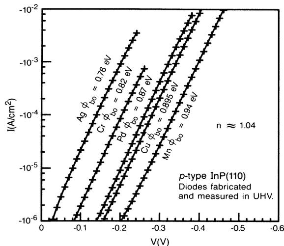
FIG. 1. An assortment of typical  $I$ - $V$  data from thick-metal diodes which were fabricated on clean cleaved  $p$ -type InP(110) surfaces and measured *in situ*. The barrier height,  $\Phi_b$  and ideality factor,  $n$  are determined from Eq. (1).
