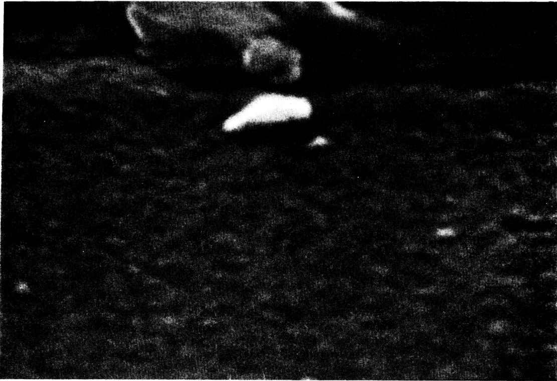
FIG. 2. Electron micrograph of a 20-nm-thick aluminum film on quartz. Observation angle is  $60^\circ$  from the normal. Debris in the upper portion of the micrograph is for focusing purposes. (Same magnification as Fig. 1).
