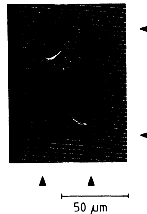
FIG. 2. Measured spatial variation of the Josephson current density in the cross-line junction sketched in Fig. 1. The beam-induced change -\delta I_{\max}(x,y) of the maximum Josephson current is plotted vertically in arbitrary units for a series of horizontal line scans ( y modulation). The triangles indicate the location of the boundaries of the junction.
