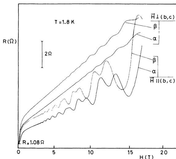
FIG. 1. Variation of the magnetoresistance of NbSe<sub>3</sub> (sample 1) at  $T = 1.8$  K with  $\mathbf{H}$  parallel and perpendicular to  $(b,c)$  plane. Curves  $\alpha$  correspond to the virgin state when the sample has just been cooled from room temperature. Curves  $\beta$  are recorded after a current (4 mA) large enough to depin the CDW has been swept up and reduced to zero.
