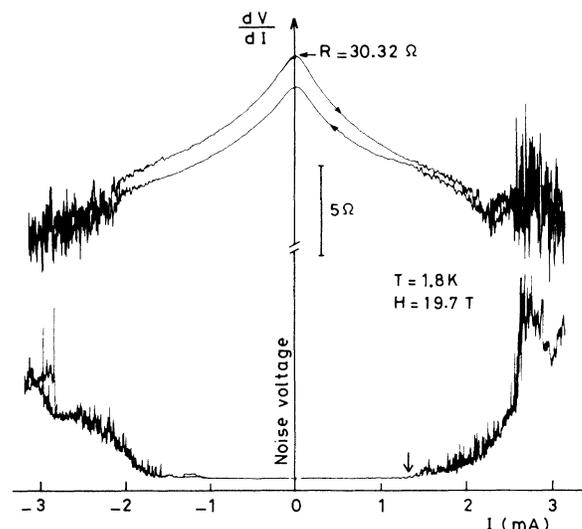
FIG. 3. Variation of the differential resistance  $dV/dI$  and of the noise voltage amplitude of NbSe<sub>3</sub> (sample 2) at  $T = 1.8$  K and  $H = 19.7$  T applied parallel to the  $(b,c)$  plane as a function of the applied current. The conductivity shows a nonlinear behavior before the noise generation and the CDW depinning.
