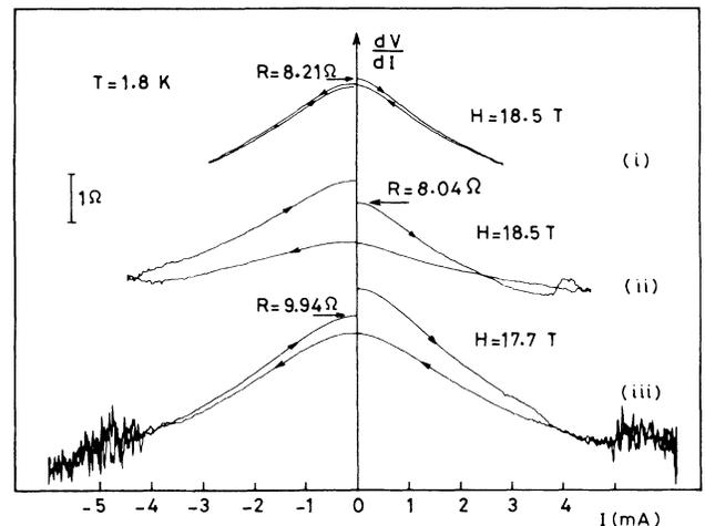
FIG. 2. Variation of the differential resistance  $dV/dI$  of NbSe<sub>3</sub> (sample 1) at  $T = 1.8$  K as a function of the applied current with  $H$  parallel to the  $(b,c)$  plane. (i)  $H = 18.5$  T and the maximum applied current (2.8 mA) does not exceed the threshold value. (ii)  $H = 18.5$  T and the CDW is depinned above 3.5 mA. (iii)  $H = 17.7$  T and with a larger current excursion.
