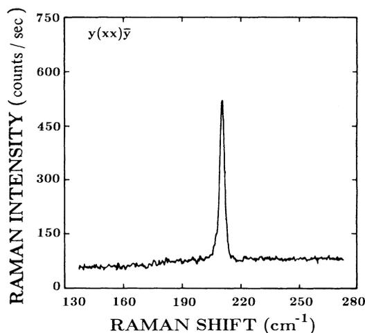
FIG. 2. Off-resonance Raman spectrum of CdSe in the  $y(xx)\bar{y}$  configuration. Energy of the exciting radiation is 1.8857 eV which is much higher than the  $A$  and  $B$  exciton energies.
