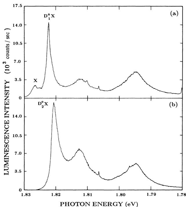
FIG. 5. Luminescence spectra of CdSe excited with the 6764 Å line of the Kr<sup>+</sup> laser. Incident polarization is perpendicular to the *c* axis. Emitted polarization is (a) perpendicular and (b) parallel to the *c* axis. The peak labeled *X* is due to free exciton.  $D_1^0X$  and  $D_2^0X$  are attributed to excitons bound to donors  $D_1$  and  $D_2$ , respectively. The peaks at 1.8127 and 1.7947 eV are assigned to donor luminescences.
