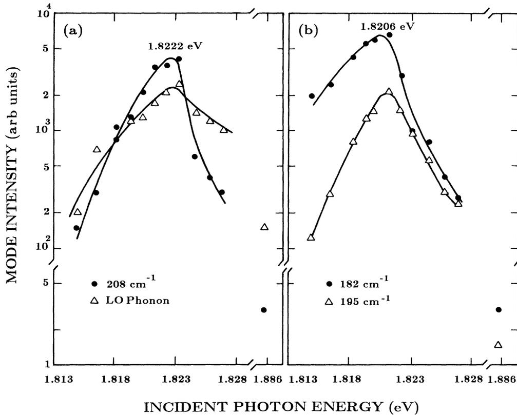
FIG. 4. Resonance enhancement of Raman intensities of the new Raman lines and that of the LO phonon in CdSe. Intensities of the modes away from resonance are also shown for the sake of comparison. The LO phonon and the mode at  $208\text{ cm}^{-1}$  show a peak at  $1.8222\text{ eV}$ , whereas modes at  $182$  and  $195\text{ cm}^{-1}$  have maximum intensity at  $1.8206\text{ eV}$ . Curves drawn through the points are only guides to the eye.
