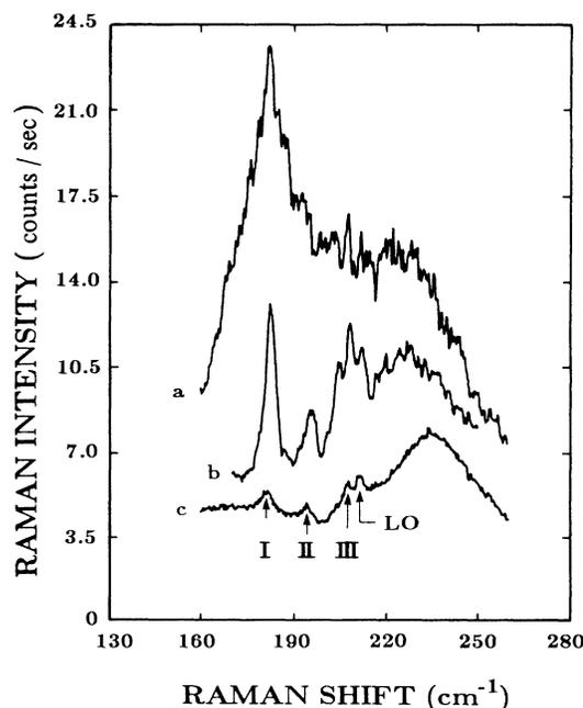
FIG. 3. Resonance Raman scattering from CdSe with the dye laser frequency tuned close to  $A$  exciton. New Raman peaks are seen at 182 (I), 195 (II), and 208 (III)  $\text{cm}^{-1}$ . Energies of the exciting radiation are (a) 1.8183, (b) 1.8211, and (c) 1.8246 eV.
