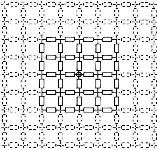
FIG. 1. Moving average window of size  $5 \times 5$  nodes. The power value assigned to the node marked with a circle is obtained by summing over all resistors denoted by solid lines.
