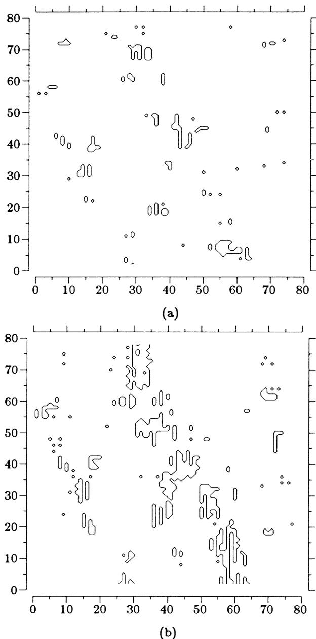
FIG. 7. Hot spot distribution after one cycle (a), and after two cycles (b), respectively, when the sample in Fig. 2 has been changed by making all hot spots well conducting. The hot spot threshold equals 1.5 times the average power density of the sample in Fig. 2.
