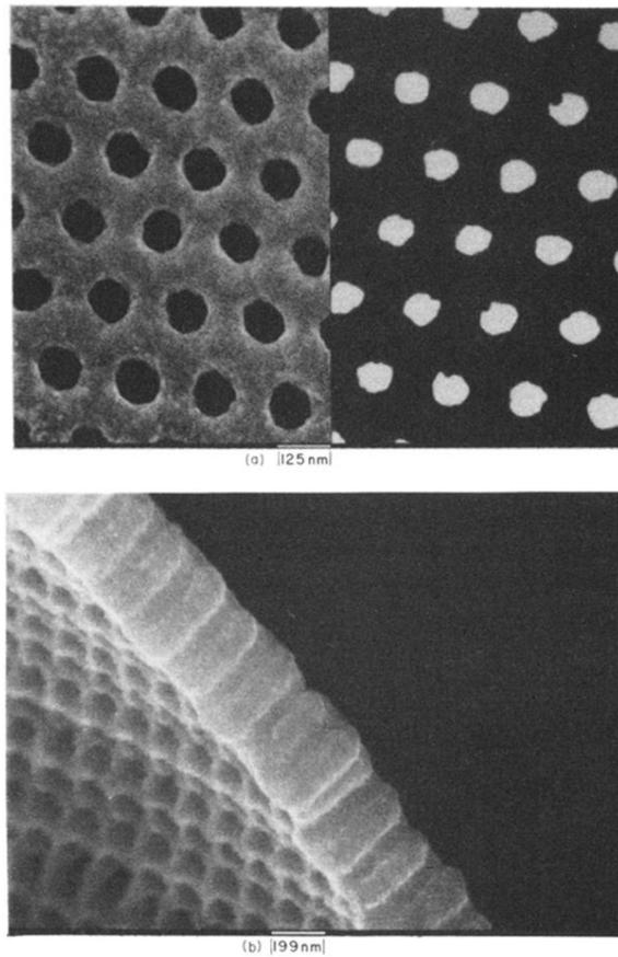
FIG. 1. Scanning electron micrographs of silver films containing microchannels. (a) A small section of a microchannel array. The frame on the right was taken in a scanning transmission electron microscope mode; the light areas are images of the transmission through the channels pictured on the left. The bar indicates a length of 125 nm. (b) A section of a torn foil sample showing part of a microchannel array as well as a number of channels in cross section. The bar indicates a length of 199 nm.
