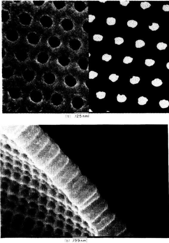
FIG. 1. Scanning electron micrographs of silver films containing microchannels. (a) A small section of a microchannel array. The frame on the right was taken in a scanning transmission electron microscope mode; the light areas are images of the transmission through the channels pictured on the left. The bar indicates a length of 125 nm. (b) A section of a torn foil sample showing part of a microchannel array as well as a number of channels in cross section. The bar indicates a length of 199 nm.
