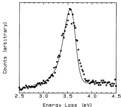
FIG. 4. Comparison of the theoretical energy-loss peak (as broadened by the energy distribution of the incident beam) with the measured peak for aloof-scattered 900-eV electrons. Circles: experimental results; solid line: theoretical results.
