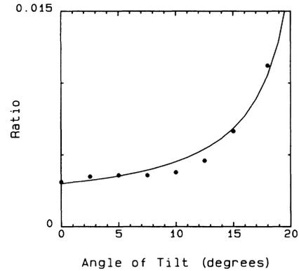
FIG. 3. Ratio of area under electron energy-loss peak to the incident flux as a function of angle between microchannel axes and direction of incident beam. Circles: experimental results; solid line: theoretical results.
