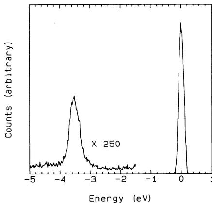
FIG. 2. Electron energy spectrum for 900-eV electrons transmitted through 100-nm-diam microchannels in a silver foil. (Beam parallel to channel axes.) The abscissa has been shifted so that the incident energy is at 0 eV.
